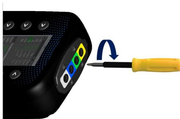
Figure 19 – Inlet Port Plate Fitting
