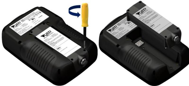
Figure 9 – Battery Removal
