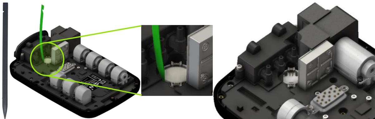
Figure 15 – Coin Cell Removed
