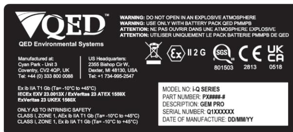
Figure 1 – i-Q Series Marking Plate
