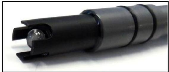
You can choose a two- or three-point pH calibration. The two-point calibration is most common, using a pH 7 buffer and a pH 4 buffer if expected values are below 7 or pH 10 buffer if expected values are above 7. If you are measuring in waters whose pH might range both above and below seven, you can increase your accuracy slightly by choosing a three-point calibration (the third buffer should be on the other side of seven). To calibrate pH:
