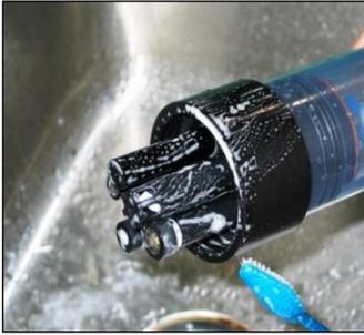
Clean your instrument periodically with warm soapy water. Clean sensor stems with a soft brush. Laboratory-grade liquid detergent is preferred, but liquid dishwashing soap is fine. Do not use abrasives. Do not use solvents such as acetone. Do not clean with gasoline, kerosene, or industrial cleaners. Rinse sensors free of soap with tap water and store the sensors in tap water (see below).
