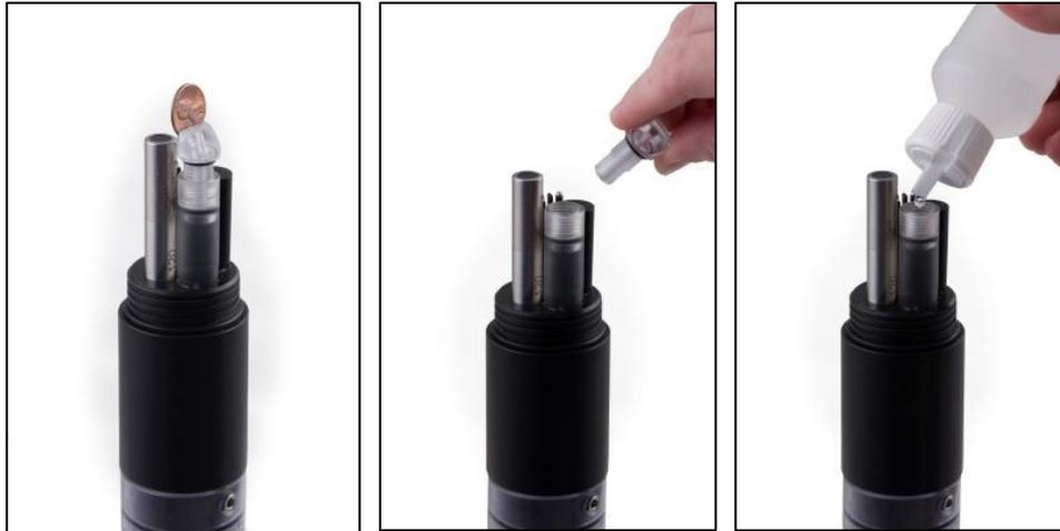
3. Screw the reference cap back on to the sleeve. As you screw the sleeve into place, air and excess electrolyte is forced out of the sleeve through the reference electrode junction (the white, porous circle at the end of the sleeve). This not only purges bubbles from the electrolyte, but also displaces any lodged particles or biological growth out of the junction.
