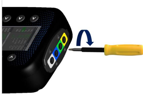
Figure 21 – Inlet Port Plate Fitting
