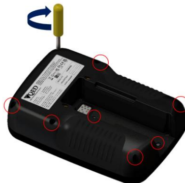
Figure 20 – Case Back Fitting
