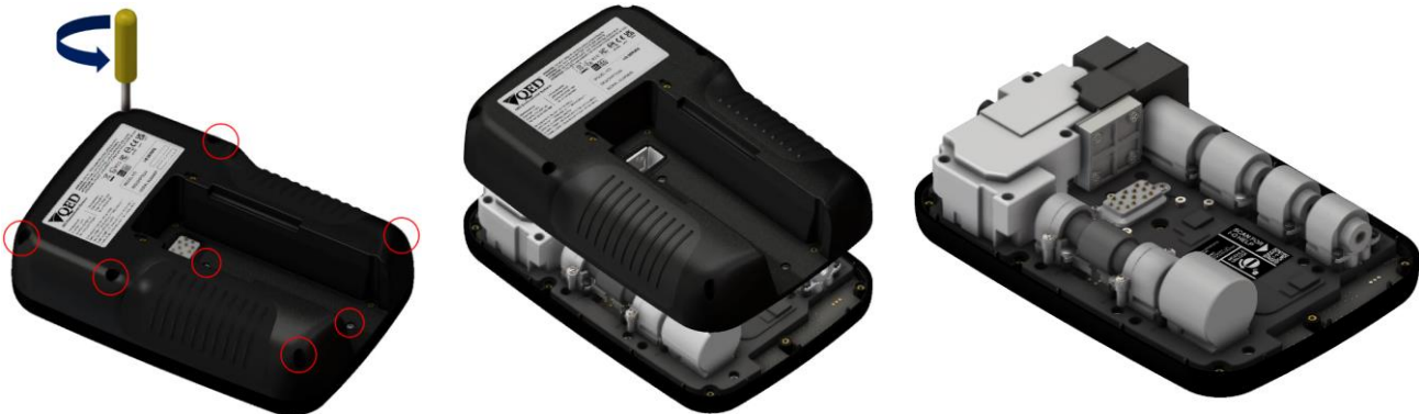
Figure 13 – Case Back Removal
