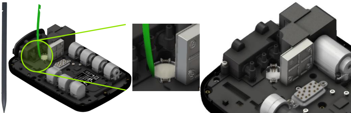
Figure 17 – Coin Cell Removed
